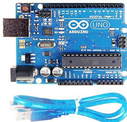
**Figure 4:** Arduino Board
